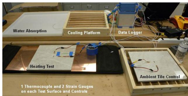
was done to ensure no liquid water contacted the strain gauges. The tile was submerged for over three hours and the strain data recorded.
