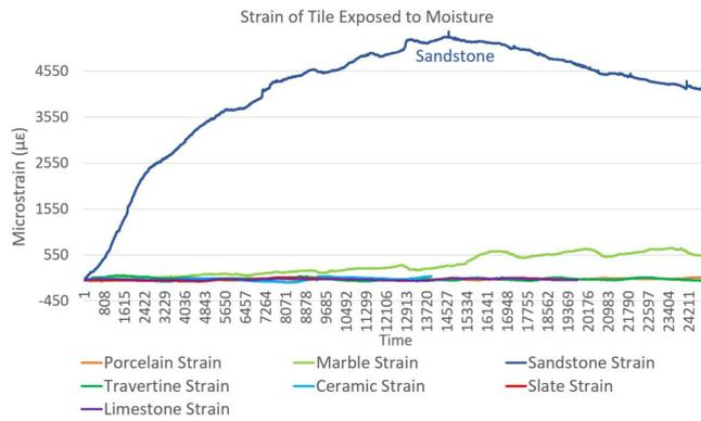
Diagram 2: Strain when exposed to liquid water (minus sandstone), marble exhibited excess strain (yellow line).
